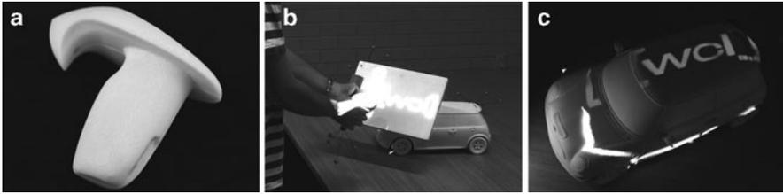
**Fig. 10.3** Digital airbrushing with SAR. (a) The airbrush tool. (b) Using a virtual stencil to paint a model car. (c) Airbrushing result
