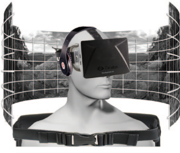
Fig. 1. Virtual reality equipment. Participants sat in supportive chairs that prevented trunk movement (i.e., a seat belt around their shoulders) and wore headphones and head-mounted displays. A 360° (cylindrical) virtual template accommodated six virtual scenes.
