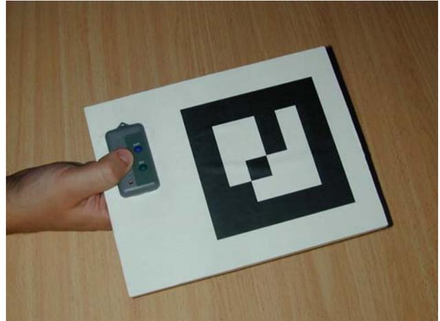
Figure 6. The wireless button enhanced fiducial marker.
