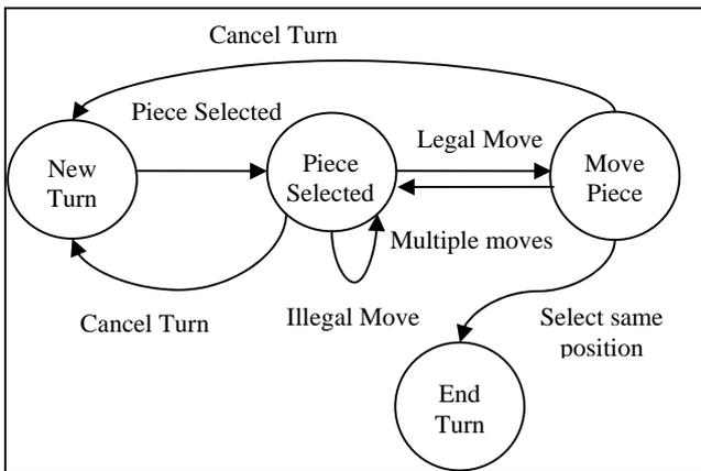
**Figure 8. The state transition diagram for a player to move one piece in Augmented Reality Chinese Checkers**
