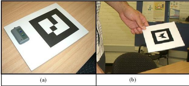
**Figure 12. (a) Button press interaction tool (b) Dwell time interaction tool**
