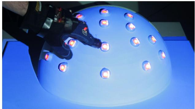
Figure 1. RFID glove used with SAR mock-up.
