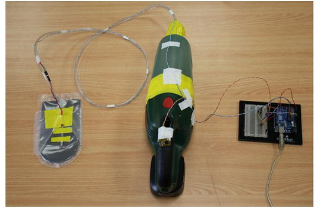
**Figure 2: Jamming system components: the jamming mitten, a vacuum pump and an Arduino microcontroller connected to a personal computer (not shown)**
