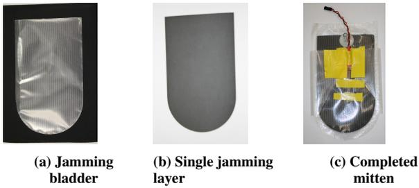
Figure 3: Components of the layer jamming mitten during construction
